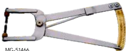
MG-51466 Measuring Gauge Has a 25mm capacity graduated in 1/4" 5mm. Highly polished nylon ball tips will not scratch plastic lenses. Heavy duty construction assures accuracy and long life. Overall length is 7 1/4" with a throat depth of 44mm.
