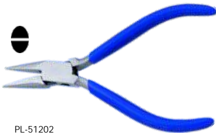
PL-51202 Chain Nose Pliers 130mm Smooth Stainless Steel Made, Box Joint without Leaf Spring, Satin Finish Pvc Handles.
