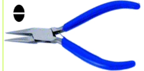
PL-51210 Chain Nose Pliers Economy 125mm Stainless Steel Made, Box Joint with Single Leaf Spring, Satin Finish Pvc Handles.
