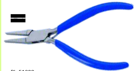
PL-51209 Flat Nose Pliers Economy 125mm Stainless Steel Made, Box Joint with Single Leaf Spring, Satin Finish Pvc Handles.
